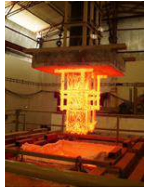
3 Fire Stop Compound just after 180 Minute Fire Test
