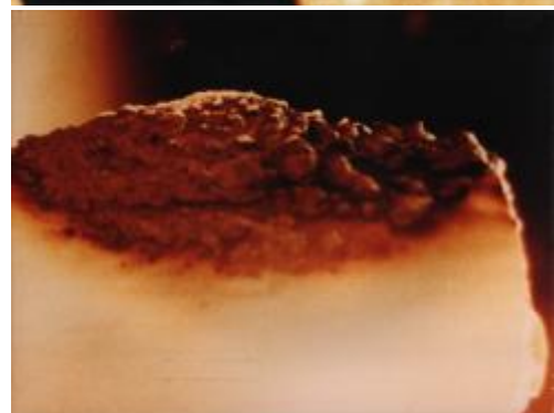
Intumescent action of Signum FR Coating on Cable
